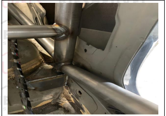
PHOTO 4 MAIN ROLLBAR TO FLOOR ATTACHMENT
