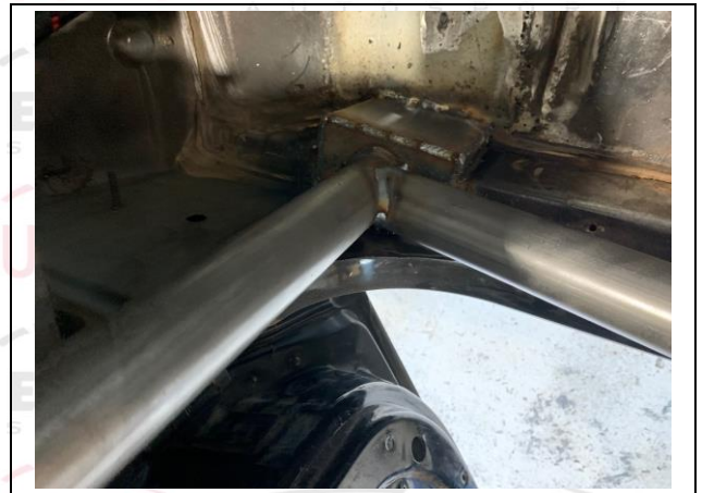
PHOTO 6 FRONT ROLLBAR TO FLOOR ATTACHMENT
